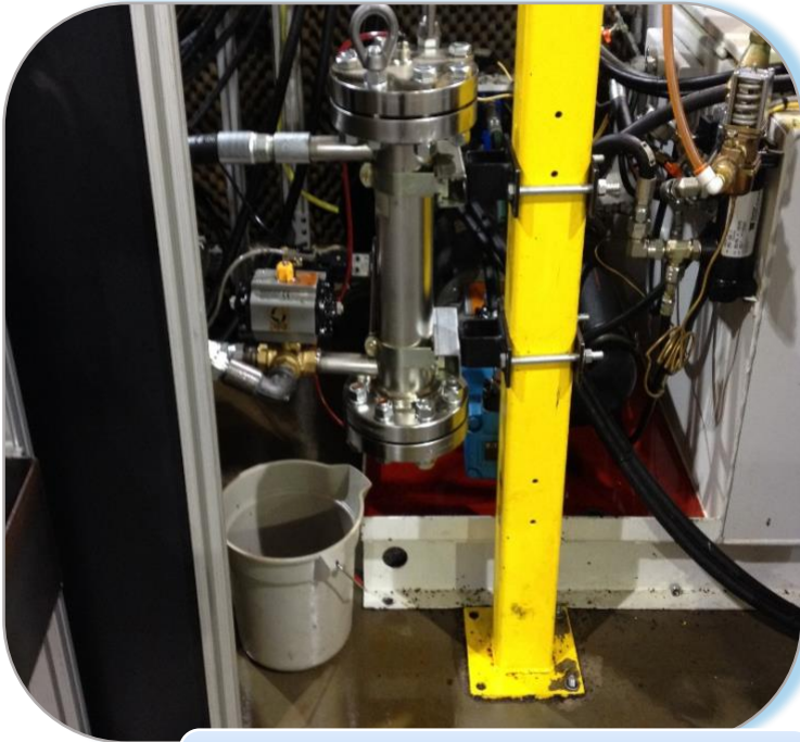
ZGF Maggie MG300 Rated at up to 25 gpm on lapping slurry
