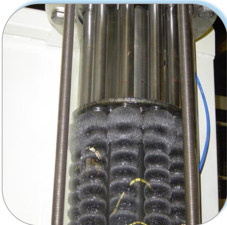
Internal View of Maggie shows steel fines captured by the powerful magnets
