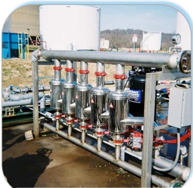
Flowrate: 800 gpm Filtration: 50 micron absolute gap
