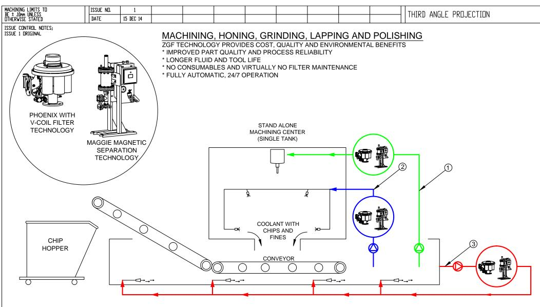
ZGF MAGGIE OR PHOENIX TECHNOLOGY CAN BE INSTALLED IN SEVERAL CRITICAL PROCESS POINTS THROUGHOUT THE SYSTEM TO PROVIDE VALUE
