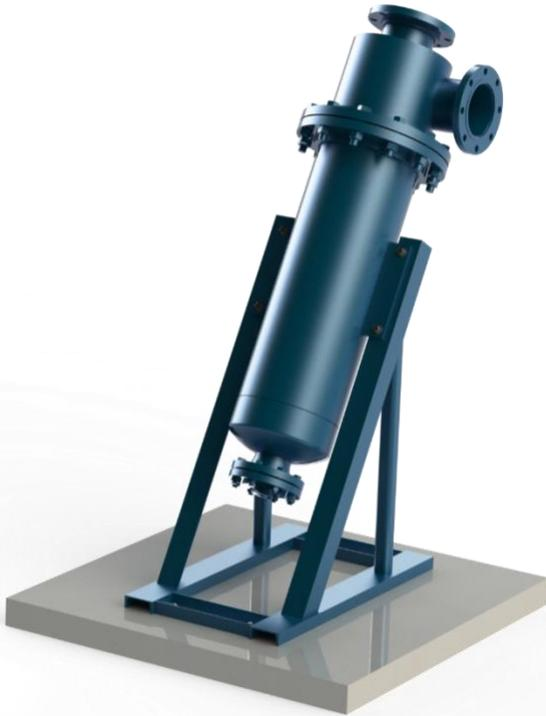
The Tornado is a patented (patent # 10,207,278) centrifugal separator that puts a new spin on an established technology! The Tornado separator is the future of centrifugal separation technology. **The innovative separator utilizes an internal blade design. The blades create a unique and beneficial flow path through the separator that increases the “G – Force” with a pressure drop of less than 1 psi, resulting in more effective and efficient particle removal with less energy consumption.**
