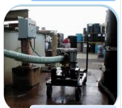
Pneumatic Phoenix Flowrate: 180 gpm Filtration: 50µ Absolute Gap
