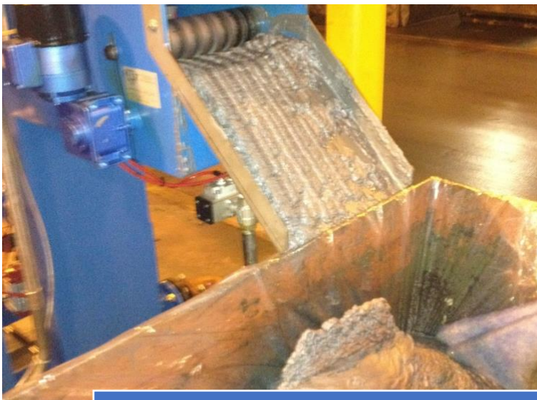
Maggie captures most particles 5 micron and larger, as well as sub-miron particles. SD+ recovers and returns the valuable honing oil to the process.
