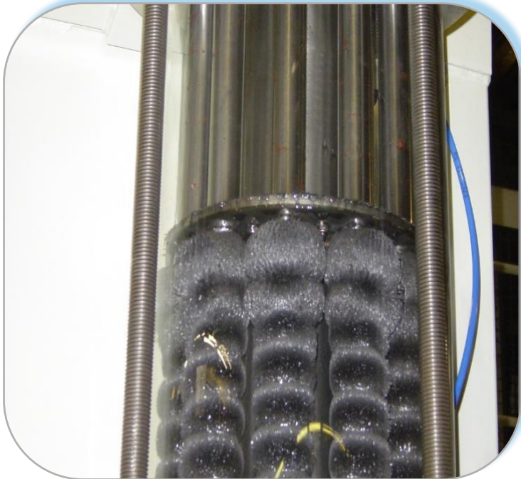
Internal View of Maggie shows ferrous scale and fines captured by the powerful magnets
