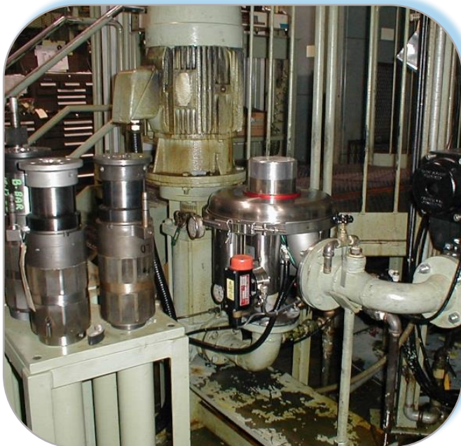
ZGF Electro-Pneumatic Phoenix provides uninterrupted flow of clean machining coolant to the tools
