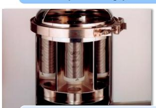
ZGF EC700S Pod cutaway view to show how elements are configured in pod
