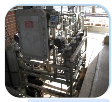
(2) x ZGF EZ Clean EC100, 4-Pod Explosion Proof Design Flow / System: 30 gpm Operating Pressure: 300psi
