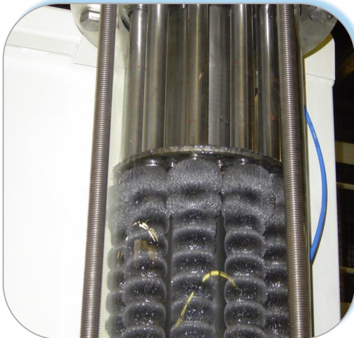
Internal View of Maggie Weld Balls & Metal Fines Captured by Maggie
