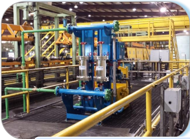
ZGF Maggie MG1200, 2-Station with Smart Drum PLUS rated at 250 gpm
