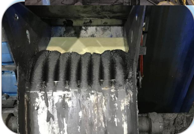
Fines and Scale Captured by Maggie and Removed by the Smart Drum PLUS
