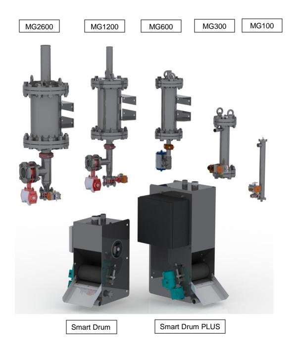
Maggie is fabricated from stainless steel. It is fully compatible with a wide range of liquids and operating conditions up to 170°F and 100 psi. Maggie is available with three standard elastomers (seals and o-rings) – Viton, Buna and EPDM. Elastomer material selection is based upon compatibility with the process fluid.
