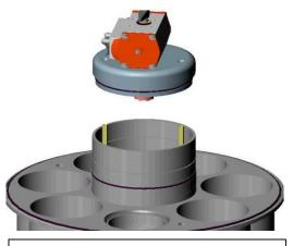
Remove control cover by lifting upwards, being careful of pneumatic airlines connected to cover.
