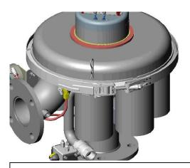
Remove safety clip from ring clamp and place in safe area.
