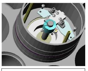
Remove either roller valve or proximity switch by removing two M4 screws holding base plate to Phoenix body.
