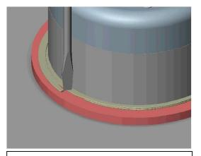
Insert flat screwdriver into tab of split retaining ring and twist. Gently lift upwards, unwinding ring from its groove.
