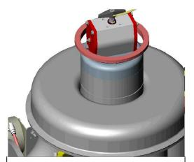
Remove red backing ring by lifting upwards.
