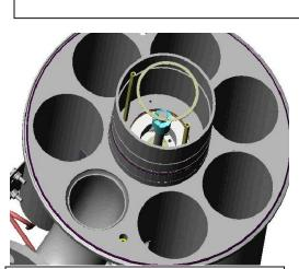
Remove valve retaining ring by inserting screwdriver into tab, twisting, and unwinding from its groove.
