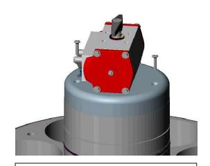
Remove two M4 screws on top of control cover. Note position of cover to filter body.
