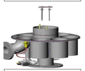
Screw valve puller (part number 9099-000) into valve body and lift upwards.
